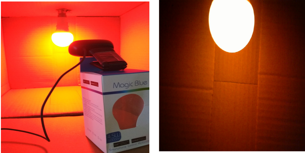
Figure 6: THE RECEIVER SETUP WHEN BULB IS SWITCHING BETWEEN MULTIPLE COLORS. THE RIGHT SIDE SHOWS THE WEBCAM VIEW IN MATLAB FOR PROCESSING THE DATA.
